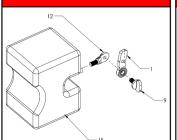
VP226 Valve VA225P Float Arm OP321 Float (Float in Vertical Position)
