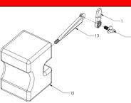
VP221 Valve WC726P Float Arm OP321 Float (Float in Vertical Position)
