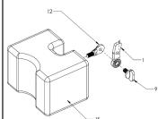
VP223 Valve VA225P Float Arm OP321 Float (Float in Horizontal Position)
