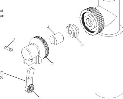
ATTENTION: DO NOT PUT PRESSURE ON VALVE ARM WHILE TIGHTENING FRONT VALVE ASSEMBLY.
