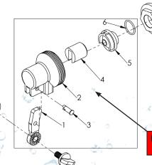
If you want to replace a VP1 valve with a VP2 valve, the base and assembly nut can remain connected to your water supply line.
