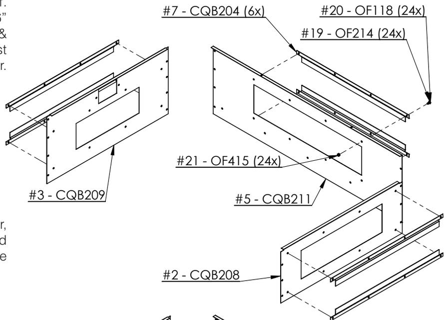
NOTE: When using all fasteners with washer, always place washer with bolt, insert bolt and washer through the part and then place on the nut.
