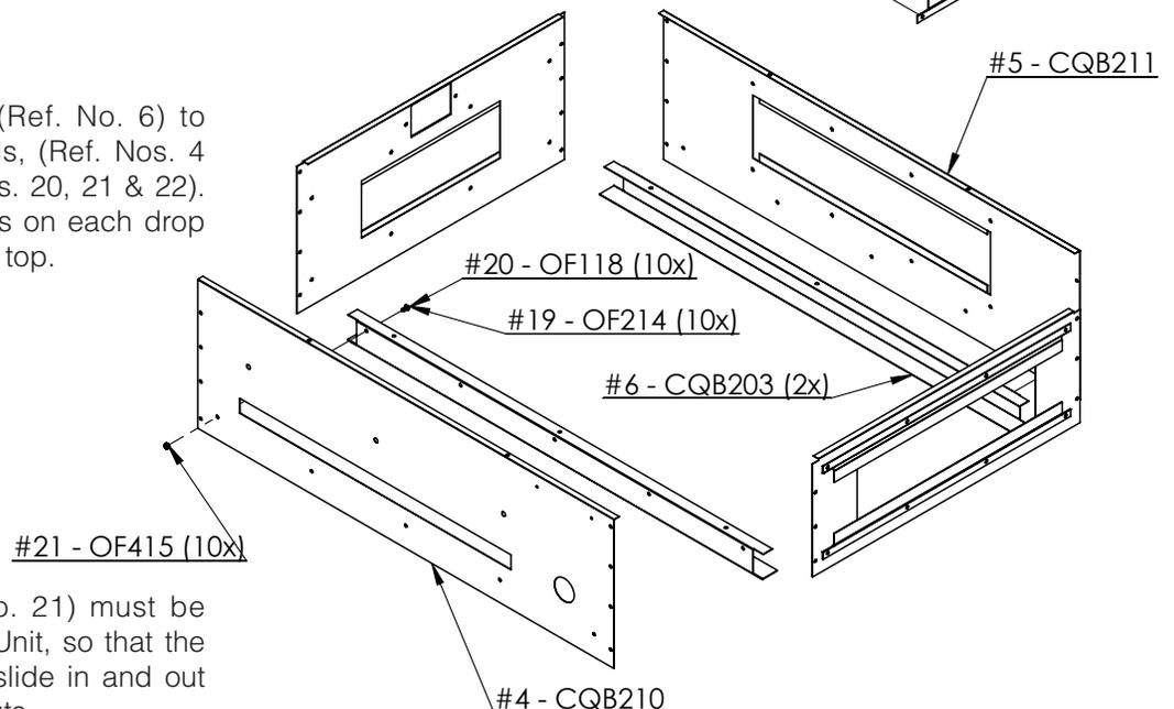
NOTE: The Locknut (Ref. No. 21) must be placed on the outside of the Unit, so that the Drop Pan (Ref. No. 13) may slide in and out after assembly. Tighten locknuts.
