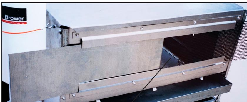
Standard are 2 sliding solid panels allowing brooder to be uniformly warm for the first few days.
